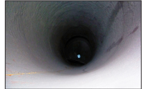
After 11 months in service minimal wear is seen to the ARC BX1*
